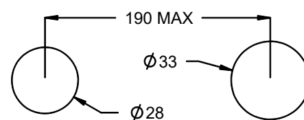
INLET BODY OUTLET ROUGH-IN DIMENSIONS
